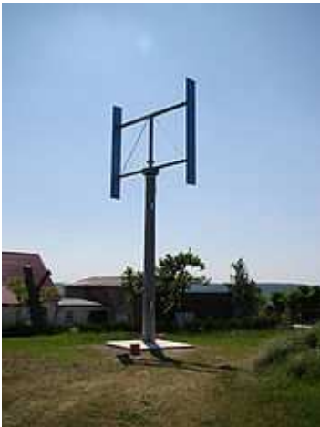
5 kilowatt vertical axis wind turbine
